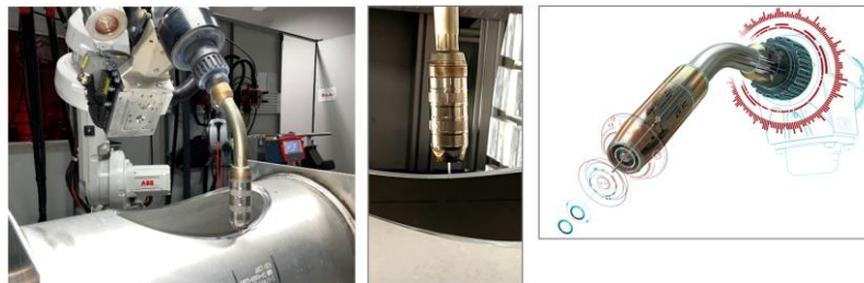
Figure 2. Wire electrode as a sensor for position and seam preparation
