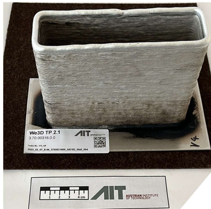
Figure 2. Reference sample of the wall geometry samples
