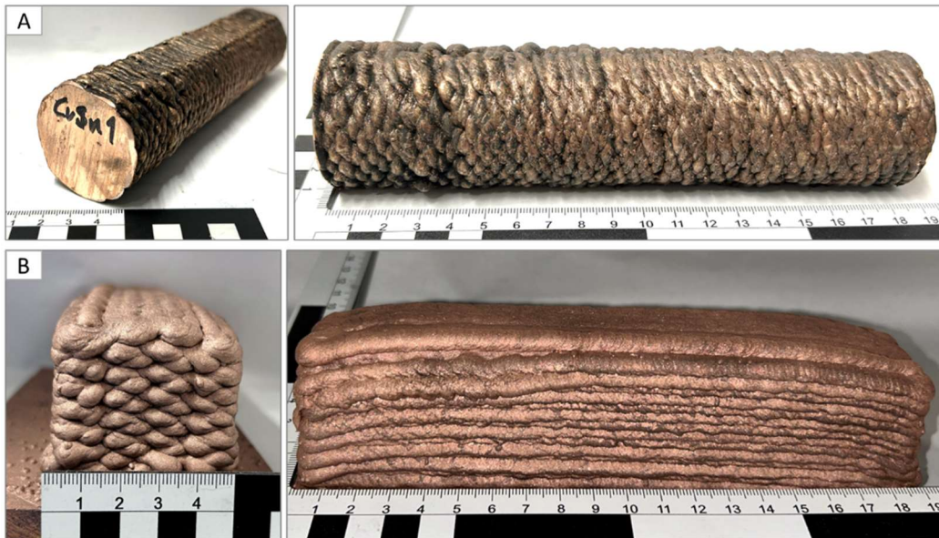
Figure 7. Solid billets (A: Vertical, B: Horizontal) produced using CuSn1 alloy.
