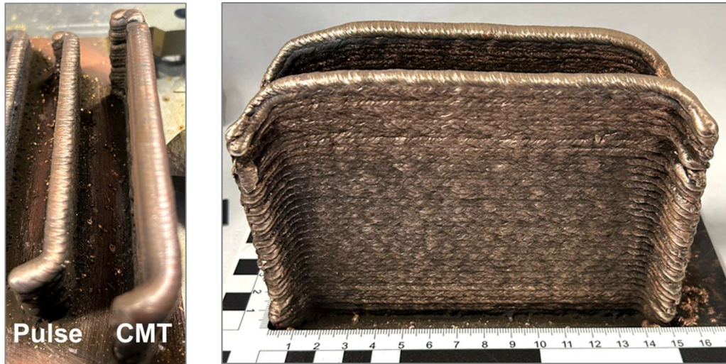
Figure 5. Walls produced with CMT and pulse WA-DED processes.
