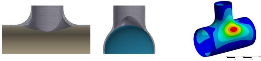
Figure 1. Additive welded transition of pipe branch and FEM model with stress concentration
