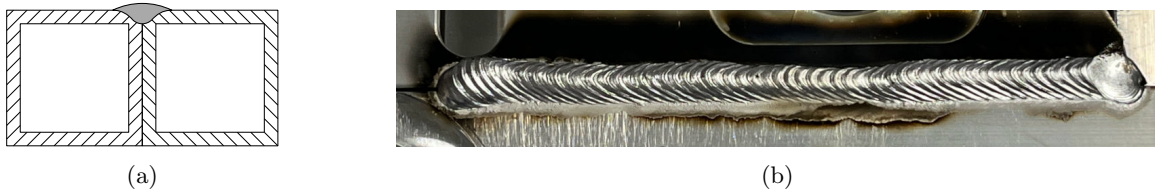
Figure 1: (a) Illustration of the cross-section and (b) photo of the weld seam.
