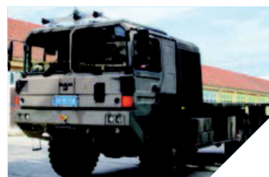
3D vision for autonomous path planning: the sensor system models the vehicle environment in 3D and generates a map.
