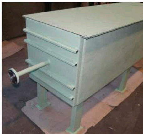
Figure 12: The final storage before it was shipped to the demonstration site including protective paint.
