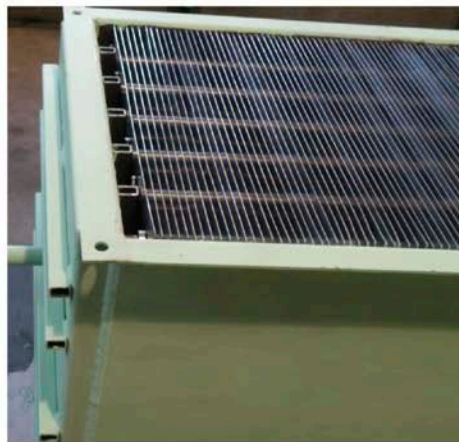
Figure 11: At the company HE Technik in Gilgenberg, Austria, the heat exchanger was welded to the collecting manifolds and a proper casing was manufactured.
