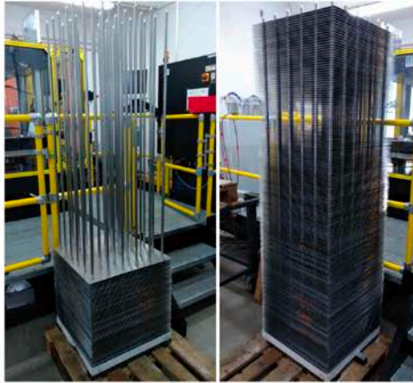
Figure 10: The heat exchanger was produced at the Light Metal Competence Center Ranshofen, Austria.
