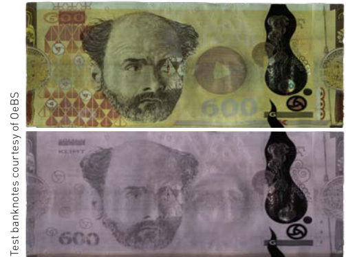
VIS (top) and NIR (bottom) data stream from a test banknote acquired with xposure with multispectral setup at 100k RGBI lines per second
