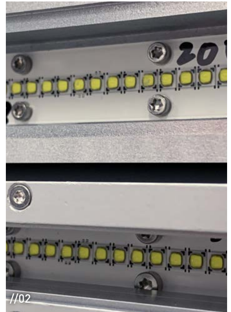
//02 xposure:flash – LED line light with 24 LEDs strobing at 600 kHz
