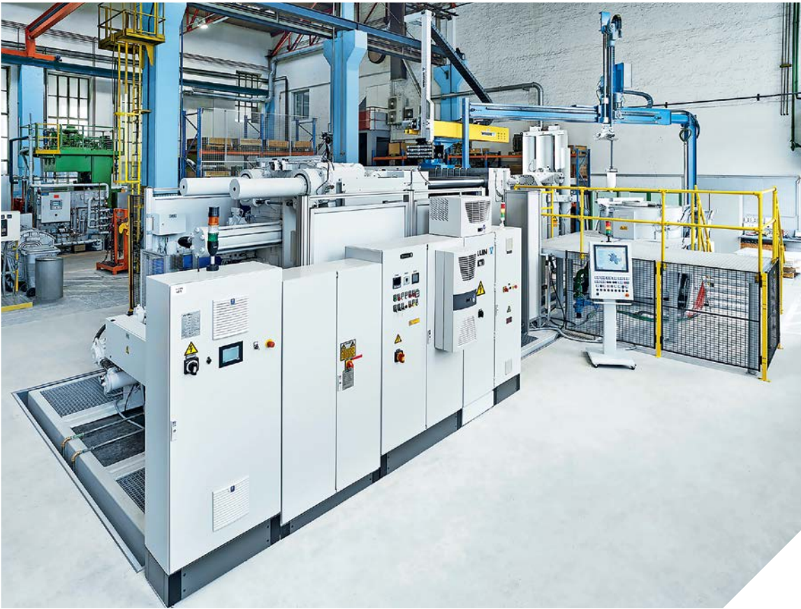
The casting machine at AIT-LKR Ranshofen: Trials on a pilot plant scale serve to optimise numerous parameters in production processes.
